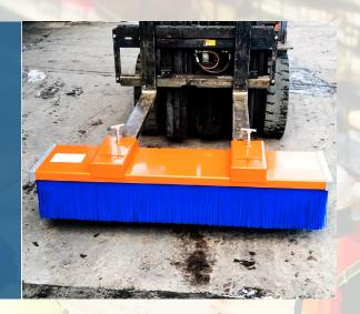
Our The Fork Mounted Sweeper is a quick and easy solution for re-heaping your loose granule products such as sand, top soil, grain or similar. Optional left and right-hand sweep gives you the versatility of clearing your yard, roadway, footpaths or warehouse.
